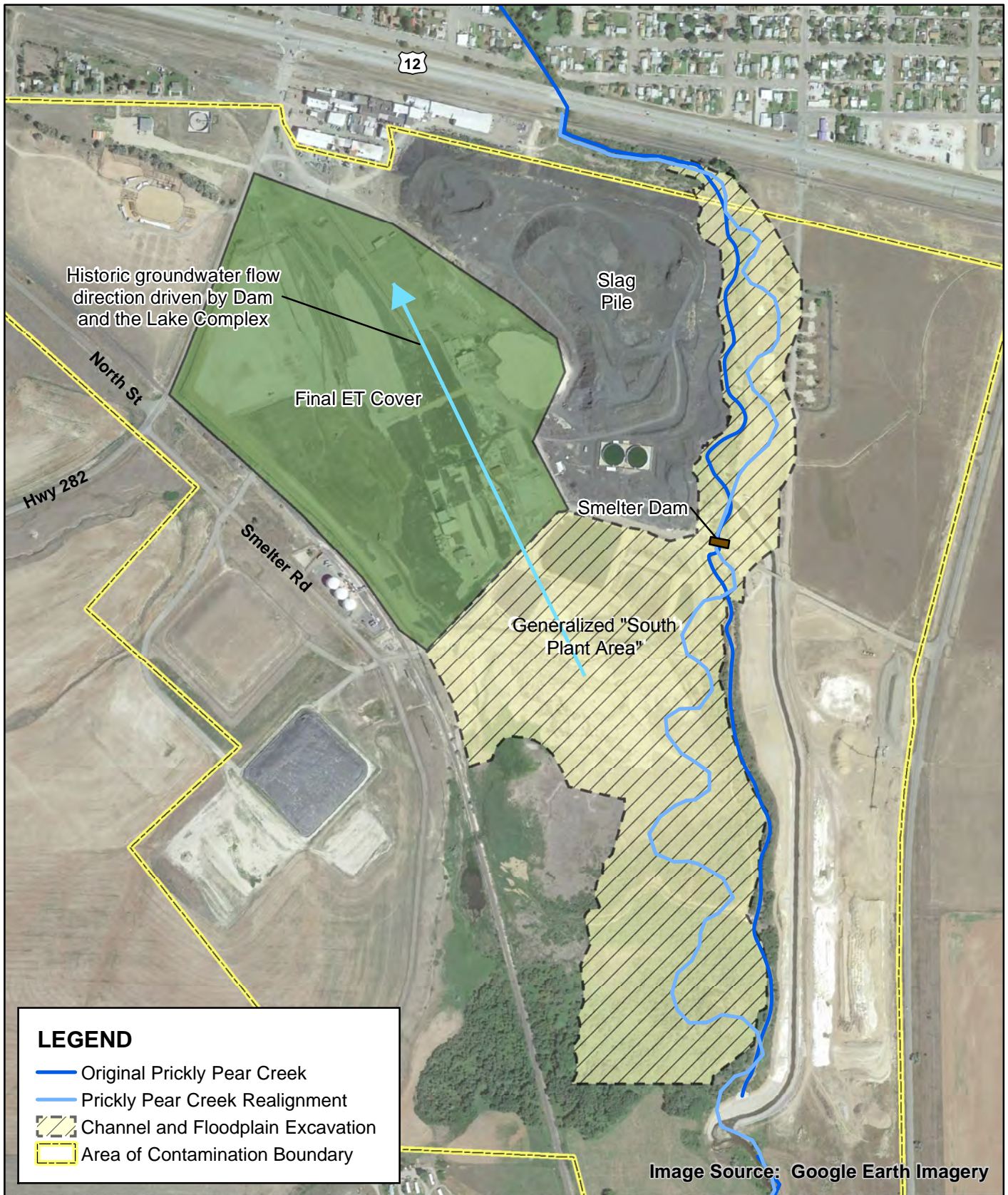
Figure 3-18 Prickly Pear Creek Realignment Former ASARCO East Helena Facility Corrective Measures Study Report East Helena, Montana
